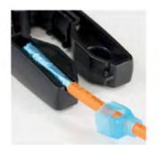
1. Insert the cable into the strain relief boot, strip off 30mm of the cable jacket, fold back the drain wire.
