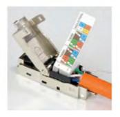
3. Remove the wiring label before placing the wire cap on the plug. Use a plier to clamp it until it completely snaps-in.
